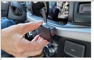
2. Insert the lower edge of the mount into the seam beneath the silver trim.
