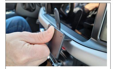
3. Press the upper part of the face plate until the mount clicks in to the opened seam on top.
